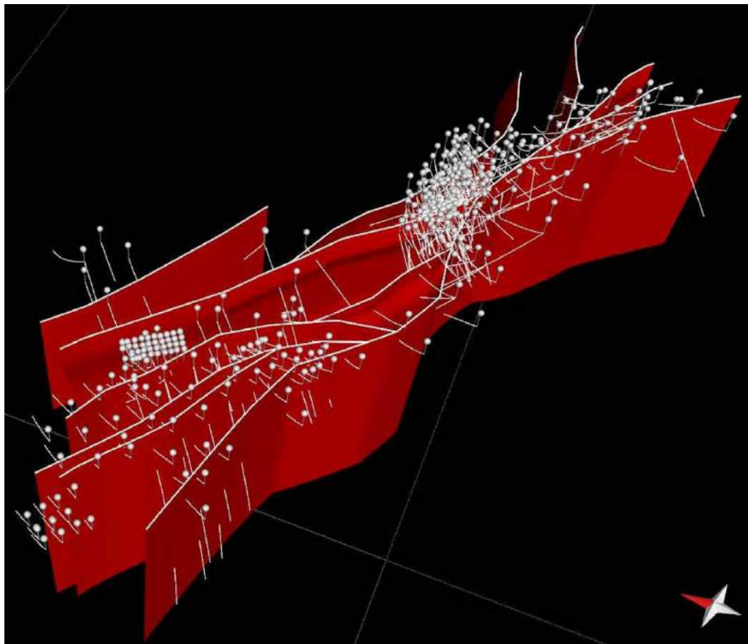
Figure 9.8 – Structural framework model of major shear zones in the Barsele area, including drill hole locations (Bauer and Imaña, 2017)
