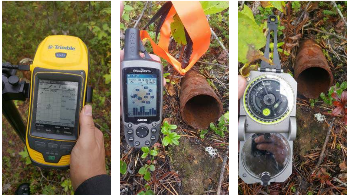
Figure 12.2 – Examples of onsite collar location verification
