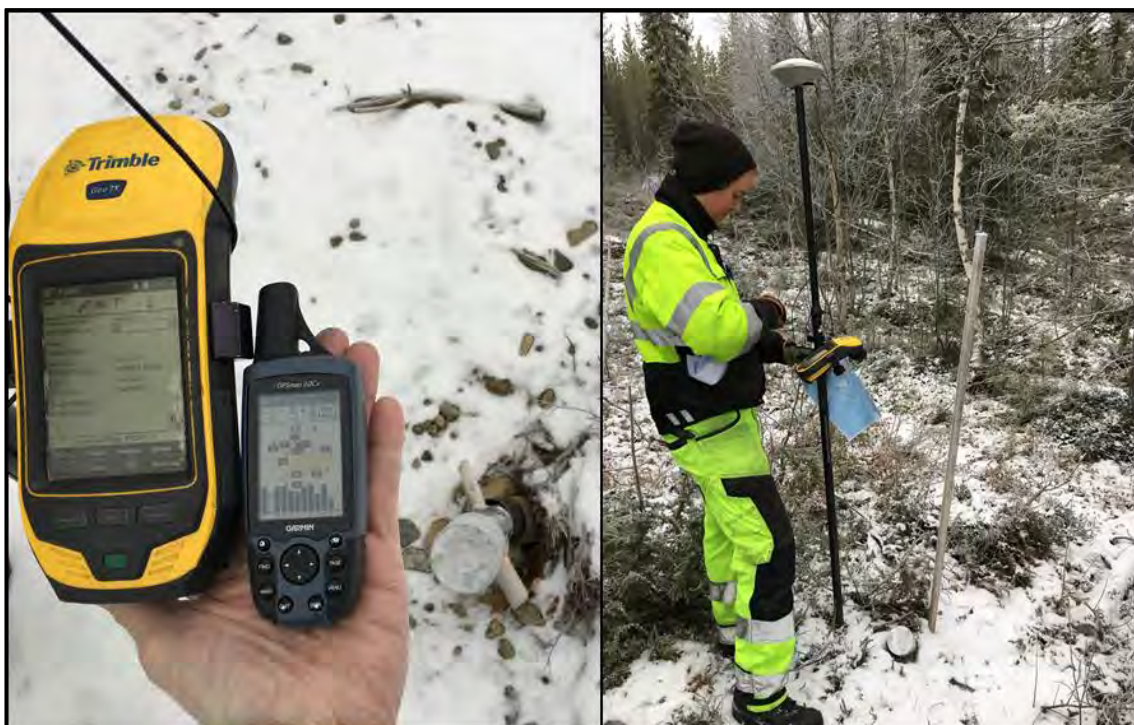
Figure 12.2 – Examples of onsite collar location verification
