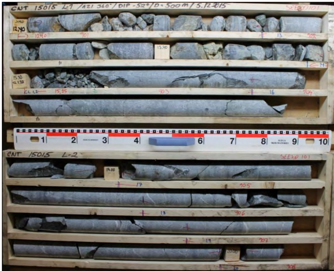
Figure 10.1 – Photography of marked drill core following the logging and sampling procedure established by AE Sweden at the Storuman core logging facility (Höglund, 2018a)
