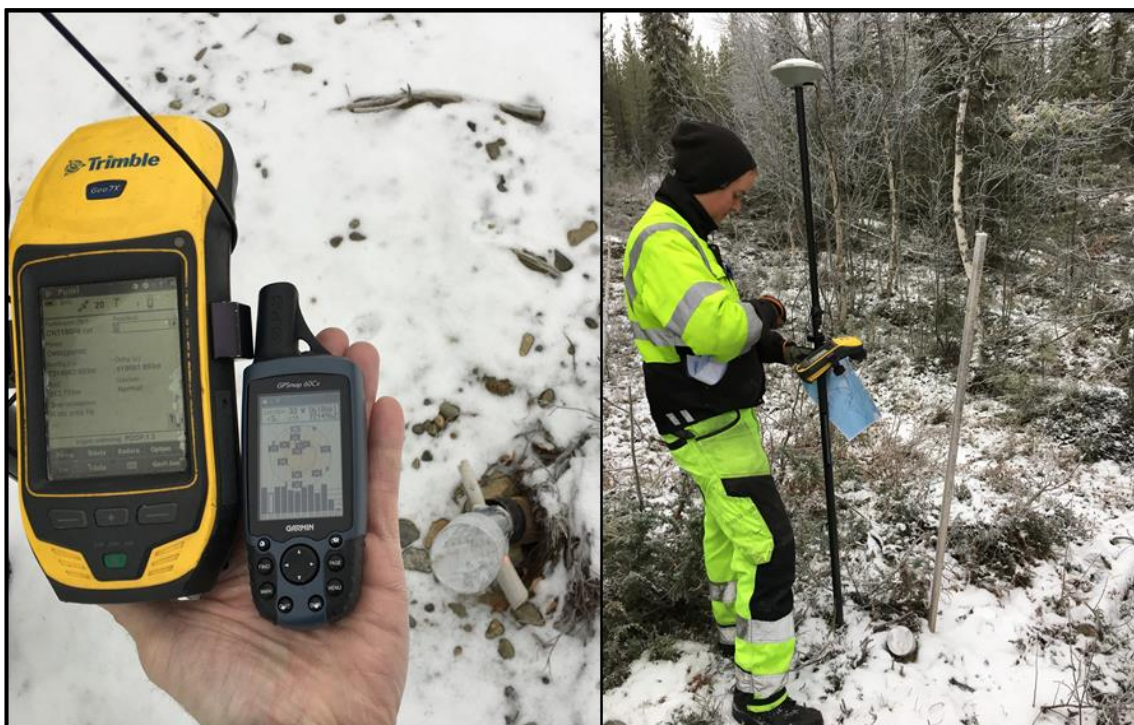
Figure 12.2 – Examples of onsite collar location verification
